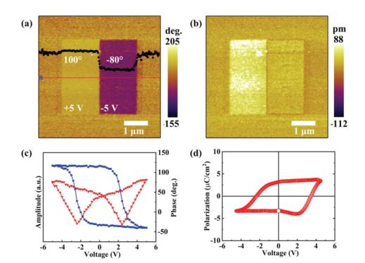
**FIG. 2.** Out-of-plane PFM phase (a) and amplitude (b) images of the HZO film, acquired after the left and right half of the central  $3\times3~\mu\mathrm{m}^2$  area was scanned with the tip biased at +5 and -5 V, respectively. The inset shows the phase of the red line, (c) switching spectroscopy PFM phase (blue) and amplitude (red) loops of the HZO film, and (d) P–V hysteresis loop of the HZO film measured at 1 kHz.
