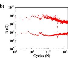
FIG. 5. (a) Retention characteristic of the Pt/HZO/Nb:STO FTJs and (b) ON and OFF resistances of the Pt/HZO/Nb:STO FTJs as functions of bipolar switching cycles.
