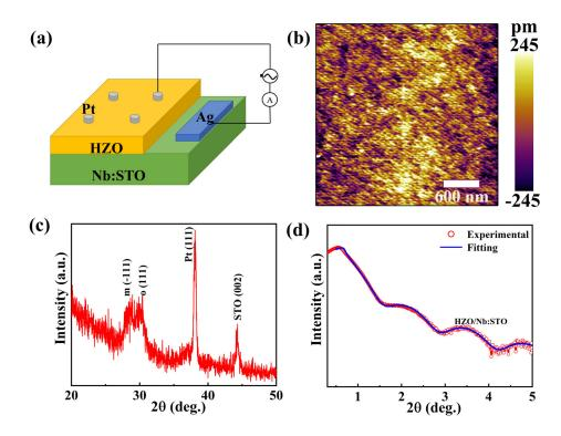
**FIG. 1.** (a) Schematic diagram of the Pt/ HZO/Nb:STO FTJs, (b) surface morphology of the HZO film over a  $3\times3~\mu\text{m}^2$  area, (c) GIXRD pattern of the Pt/HZO/Nb:STO FTJs, and (d) XRR pattern of the HZO film deposited on Nb:STO with filting
