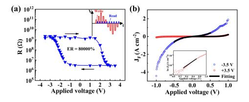
FIG. 3. (a) *R–V* hysteresis loop of the Pt/ HZO/Nb:STO FTJs. The inset shows the pulse train for the measurement and (b) *J–V* curves measured at the ON and the OFF states with fittings. The inset is  $\ln J_F - V$  curve for the ON state and its fitting with Eq. (2).
